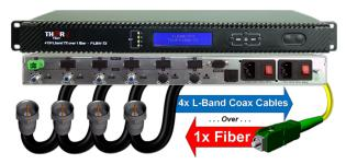
The F-LB41 platform from Thor Fiber combines four independent L-Band transmitters and receivers into a common 19 inch rackmount enclosure with dual power supplies. The power supplies can be ordered for AC or DC power, and function in hot or cold standby mode. The optics in the standard model are DWDM type lasers.
