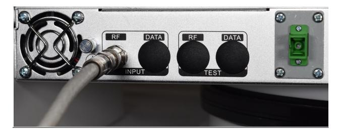
5. Connect the SC/APC jumper to the green optical port.
