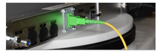
For short distance, point-to-point transmission, installing a 5db attenuator (included in the box) maybe needed inline between the transmitter and the jumper. Shown below is how to install the attenuator in series.
