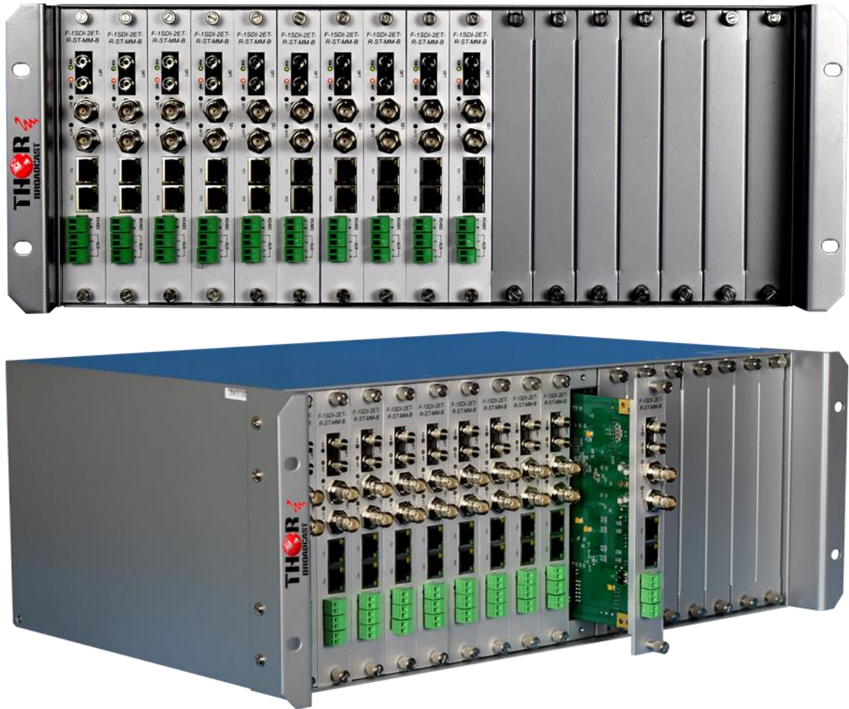
Figure 3-2-1 Rack Mount Chassis (picture with F-M1SDI-2ET-RK Cards)
