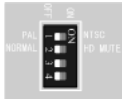
Figure 5-1 The dial switch for PAL/NTSC standard and embedded audio
