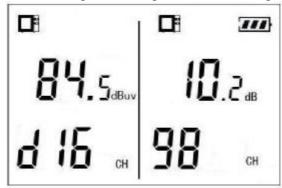
The moment the left top of the screen shows the average power level of the first digital channel, while the right top shows the difference between the average power level of the first channel and the average power level of the second channel
