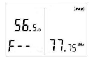
The moment, "F--" appears on the right bottom of screen, while aural carrier (or FM) frequency of the channel appears on the right bottom of the screen, and the level of aural carrier appears on the left-hand side of the screen.
