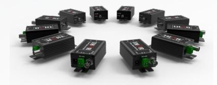
Thor F-M1SDI fiber optic SDI transmitters and receivers use locking type ST fiber connectors and BNC video cables to ensure that any cable is not accidentally pulled out of the device once the equipment is installed. Adapter jumpers are available by request for most types of fiber cables if a different fiber connector type is required. Options are available for both singlemode or multimode fiber, and a range of transmitter power options can be selected.
