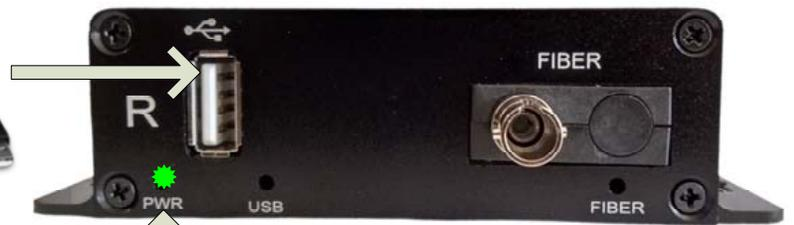
“PWR” LEDs on both T and R indicate power is properly connected
