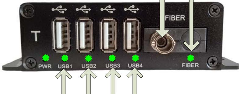
Connect USB devices to Transmitter.
