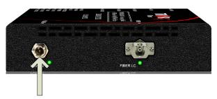
1). Connect the included DC12V Power Supplies to the TRANSMITTER (TX) and the RECEIVER (RX)
