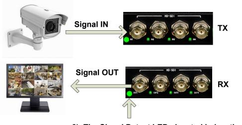
3). The Signal Detect LEDs located below the BNC connectors will light GREEN on both units once a valid SDI input signal is detected on the TX side.
