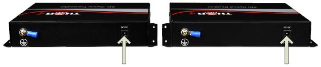
1). Connect the included DC12V Power Supplies to the TRANSMITTER (TX) and the RECEIVER (RX)
