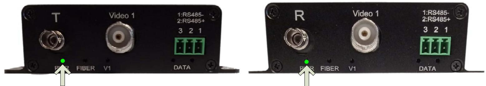
“PWR” LEDs on both T and R indicate power is properly connected
