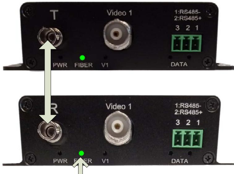
“FIBER” LEDs on both T and R indicate fiber is properly connected
