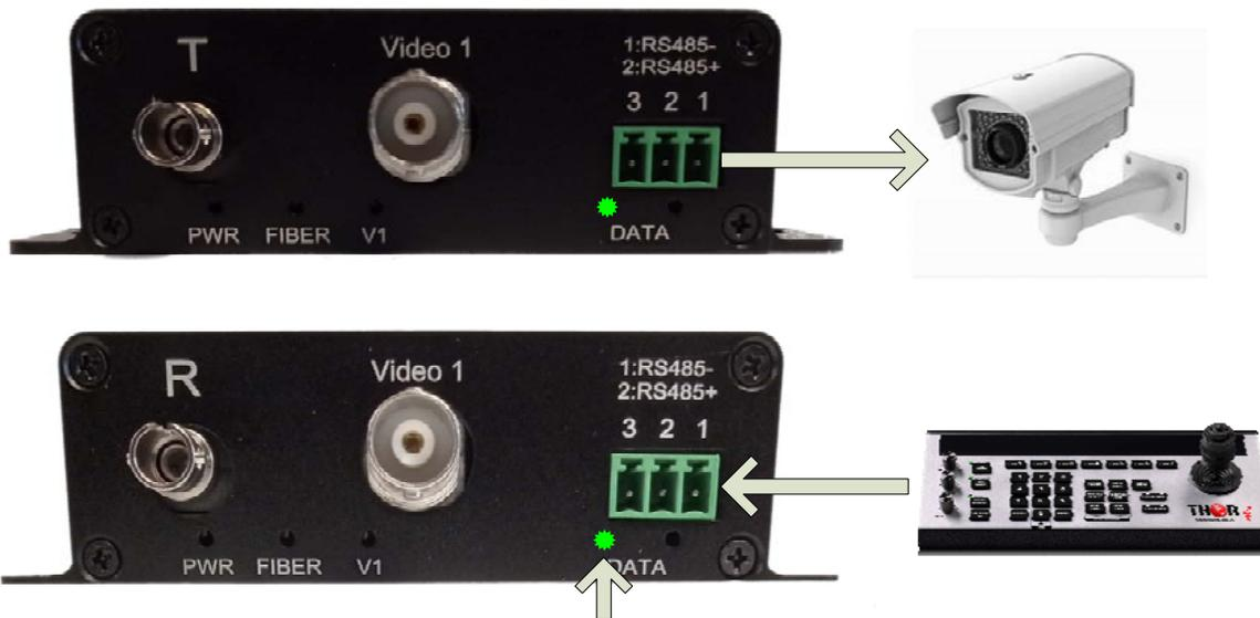
“DATA” LEDs on both T and R indicate RS data is properly connected
