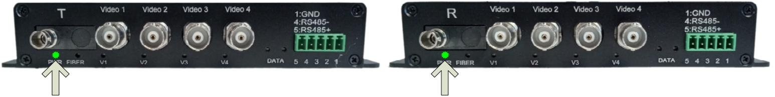
“PWR” LEDs on both T and R indicate power is properly connected
