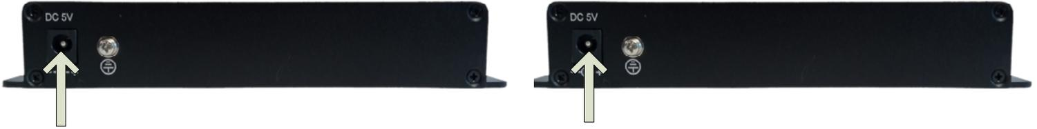
Connect Included Power Supplies to Transmitter (T) and Receiver (R)
