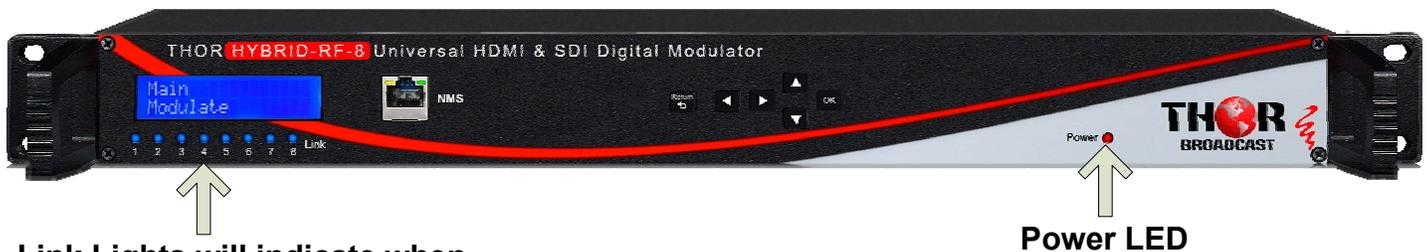
Link Lights will indicate when inputs are properly connected.
