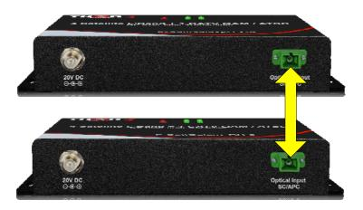
Connect Transmitter (TX) to Receiver (RX) using single mode fiber with SC APC optical connecters. (Not Included)
