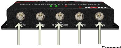
**Connect signal Input** to Transmitter (TX) and Output to Receiver (RX)
