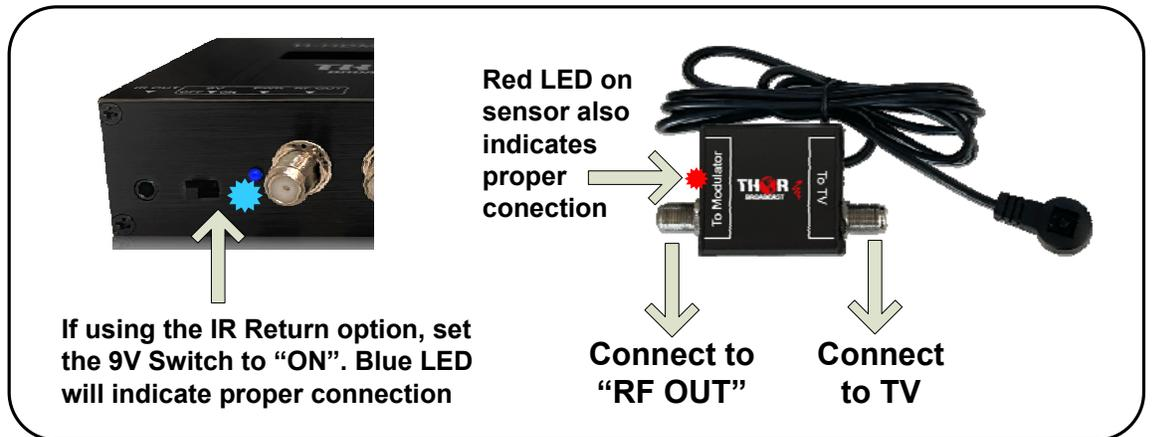
If using the IR Return option, set the 9V Switch to "ON". Blue LED will indicate proper connection
