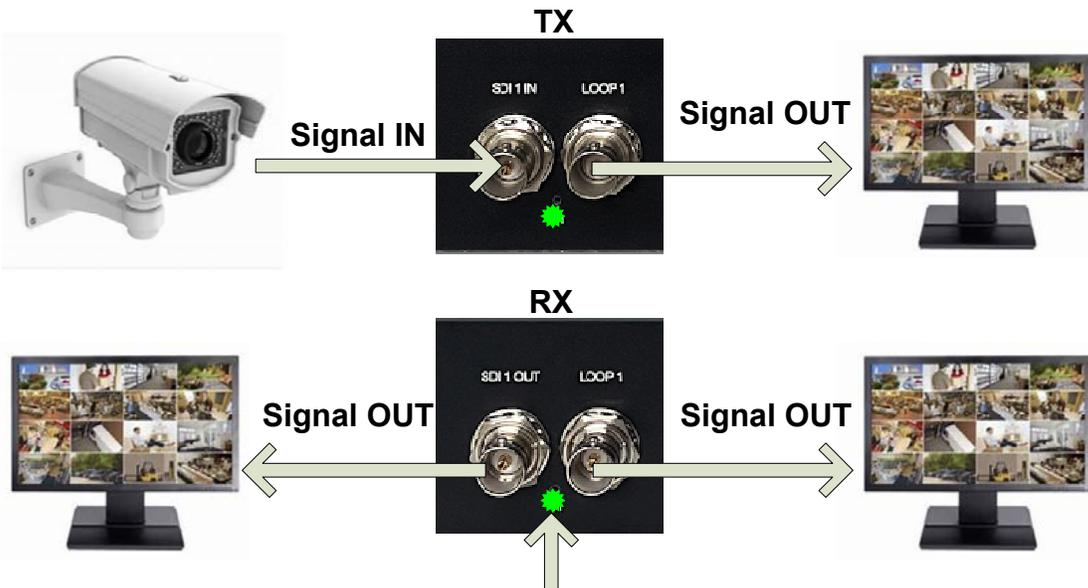
V1-V8 LEDs on both TX and RX will light GREEN when INPUT is properly connected
