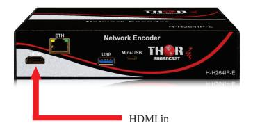
3. Connect an Ethernet cable (Cat5/6) from your computer directly into the front of your Network Encoder into the port labeled ETH. If everything is configured correctly you should see the Network Link light come on solid green on the ETH port. And momentarily you should see a communication light start blinking orange on the left. This indicates that your computer and device are communicating.
