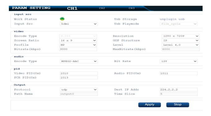
7. Click on the CH1, CH2, or CH3 tabs at the top of the page to adjust the settings for the respective channel.
