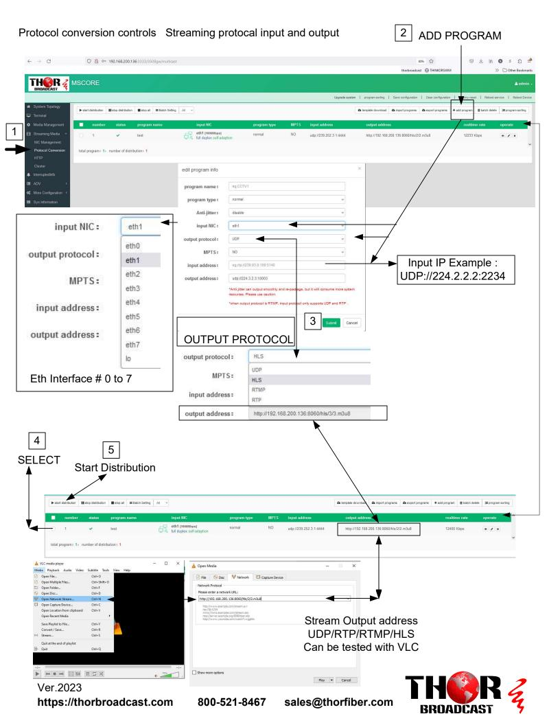
Devices have 8 Ethernet ports, and each port has its own unique IP address ranging from 192.168.200.136 to 192.168.207.136. The device's management interface can be accessed through any of these ports.
