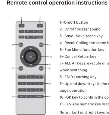
1--On/off button 2--On/off buzzer sound 3--Save Save scene key 4--Recall Calling the scene key 5--Fun Menu function key 6--Cancel Return key 7--ALL All keys, execute all switching commands when switching 8--EDID Learning Key 9--Up and down keys in the menu function can turn the page operation 10--OK key to confirm the operation 11--0-9-key numeric key area
