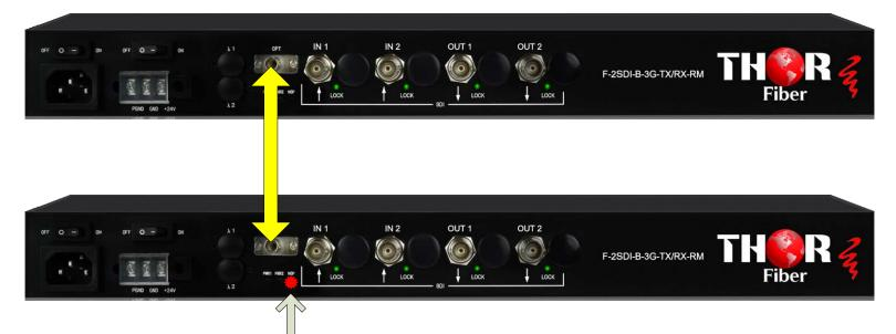
2). The 'NOP' LED will light RED only if the fiber is disconnected. When the fiber is properly connected, the 'NOP' LED will turn off.
