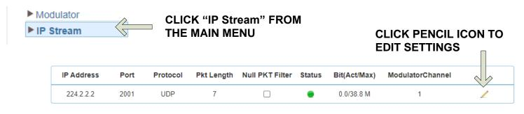
USING AN ETHERNET CABLE, CONNECT YOUR STREAMING DEVICE(S) TO PORT GE1 AND/OR GE2. ACCESS THE STREAM USING THE APPROPRIATE IP ADDRESS & PORT NUMBER:
