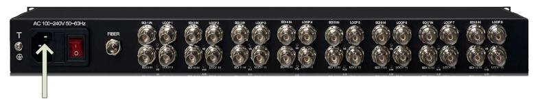
Connect Included Power Cables to both Transmitter (TX) and Receiver (RX)
