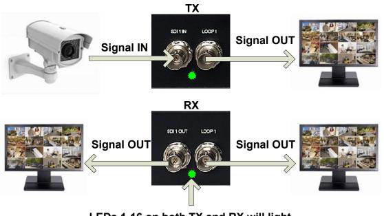
LEDs 1-16 on both TX and RX will light GREEN when INPUT is properly connected
