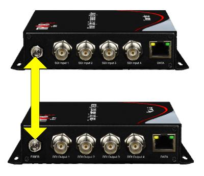
Connect a single-mode fiber optic cable between the Fiber OUT on the TX and the Fiber IN on the RX.
