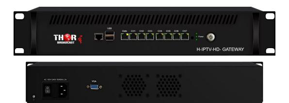
It is designed for protocol conversion and streaming media distribution applications. The unit can convert broadcast network IP streams over SRT, HTTP, UDP, RTP, RTSP, HLS, and TS file formats into SRT, HTTP, UDP, HLS, and RTMP protocols.
