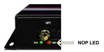
The NOP LED indicates the status of the fiber connection. It will turn off when the fiber is properly connected and light red when disconnected.
