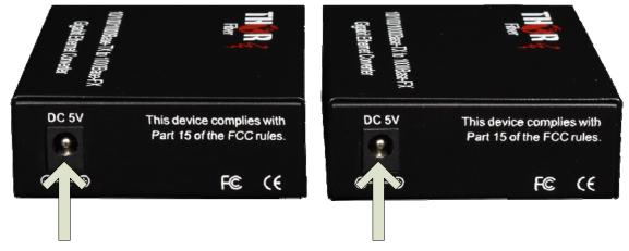
Connect included power supplies to both units A and B
