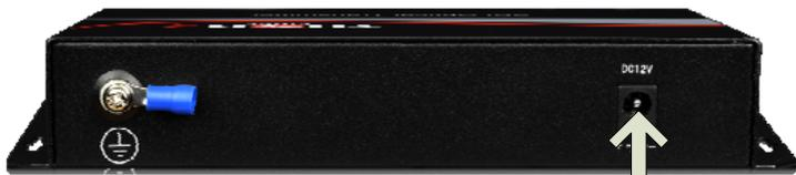
Connect the included Power Supplies to the TRANSMITTER and the RECEIVER
