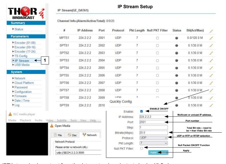
IPTV streaming is sent out from the data port and can be tested using VLC player.
