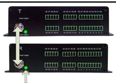
"FIBER" LEDs on both T and R indicate fiber is properly connected
