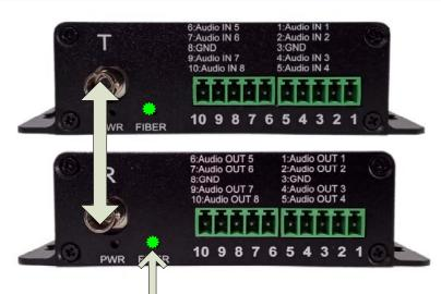
"FIBER" LEDs on both T and R indicate fiber is properly connected
