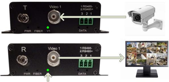
"V1" LEDs on both T and R indicate video is properly connected
