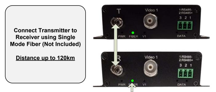
"FIBER" LEDs on both T and R indicate fiber is properly connected
