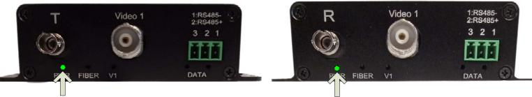
"PWR" LEDs on both T and R indicate power is properly connected
