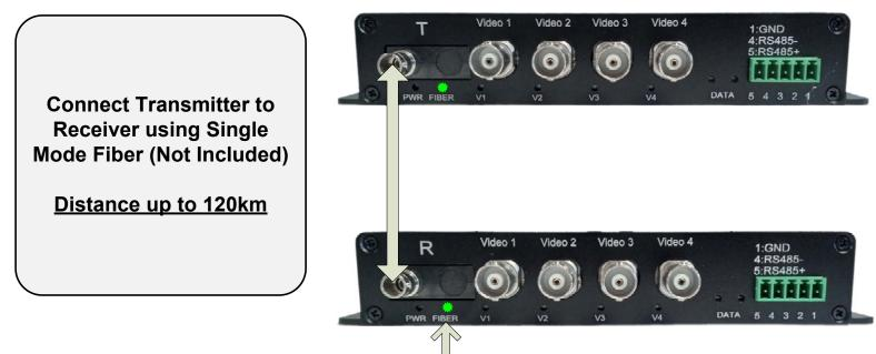
"FIBER" LEDs on both T and R indicate fiber is properly connected
