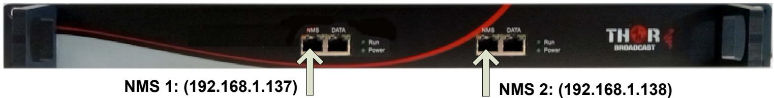
Connect the NMS port to your PC using an Ethernet cable
