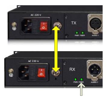
Connect Transmitter to Receiver using Single Mode Fiber (Not Included) ST/PC fiber connector
