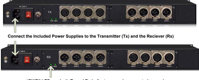
"PWR" LEDs on both Tx and Rx indicate power is connected properly
