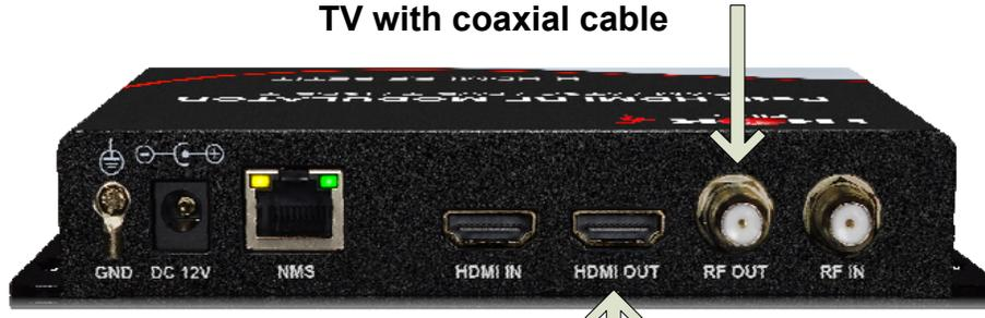
Optionally, you can connect to your TV using the HDMI OUT as a pass-through port
