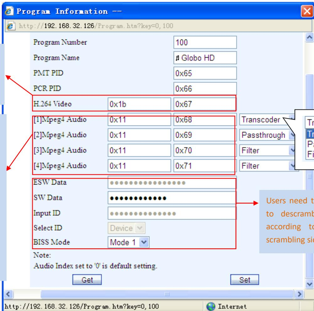
Target video format and PID can be set here:
