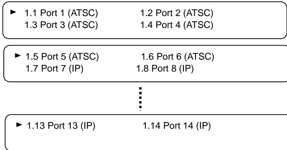
There are 6 pages displaying menus from 1.1 to 1.16 to represent the **6 tuner inputs (1.1-1.6)** and **8 IP channels (1.7-1.14)**. User can enter each sub-menu to configure its parameters.
