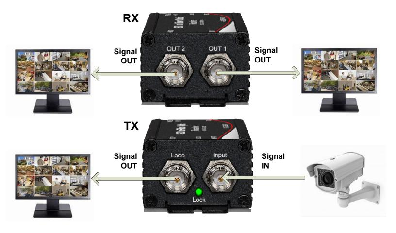
4). The "Lock" LEDs on both units will light GREEN when a valid SDI signal is detected on the TX INPUT.
