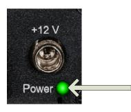
2). Power indicator LEDs on both the TX and RX will light GREEN when the units are receiving power.
