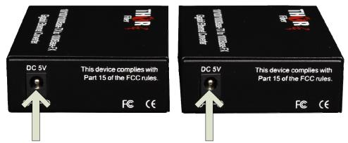
1). Connect included DC5V power supplies to both units A and B
