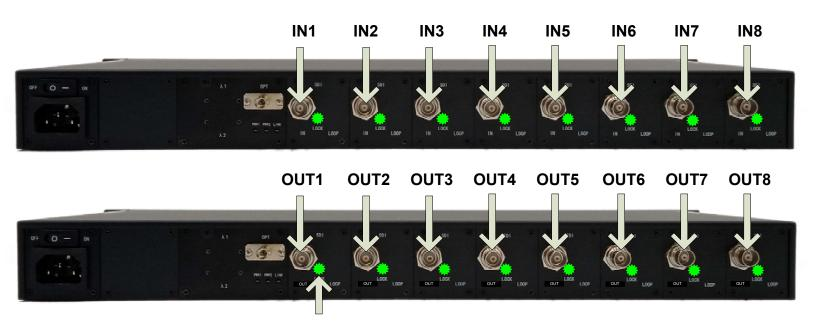
"LOCK" LEDs on both TX and RX will light GREEN indicating video is properly connected
