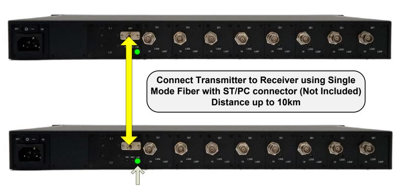
"LINK" LED will light GREEN on both TX and RX when fiber is properly connected. RX LINK LED will light RED when fiber is not connected.
